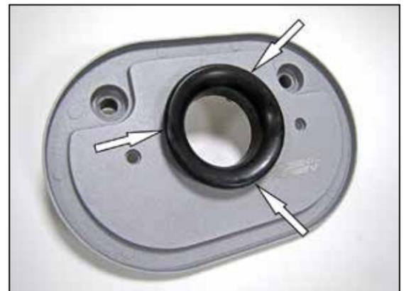
7. Install the provided intake velocity stack and the three throttle body bolts in the K&N® back plate.
