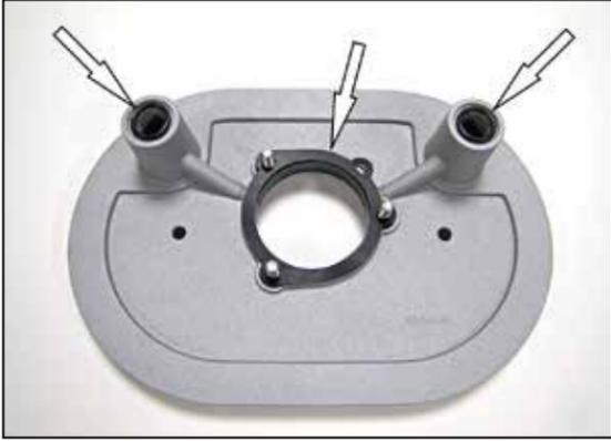
9. Install the remaining two O rings and the two filter spacers onto the front of the K&N® back plate as shown using the provided hardware.
