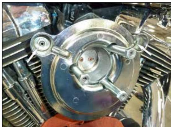
5. Remove the two rubber vent adapters from the vent bolts and then remove the two vent bolts.
