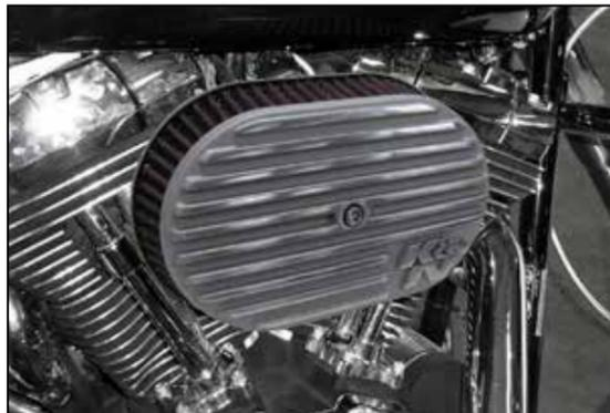
12. Attach cover plate with provided socket head Allen screw.
