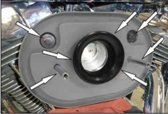
10. Install the two provided standoffs onto the filter back plate, then install the filter back plate onto the throttle body and secure first with the throttle body bolts and then with the breather bolts.
