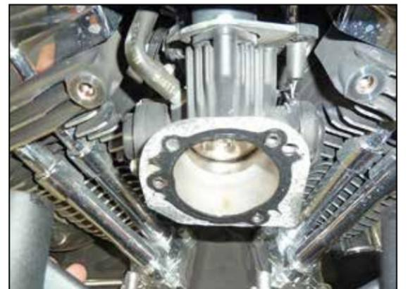
6. Remove the backing plate and stock gasket. **NOTE: K&N Engineering, Inc. recommends that customers do not discard the factory air intake components.**
