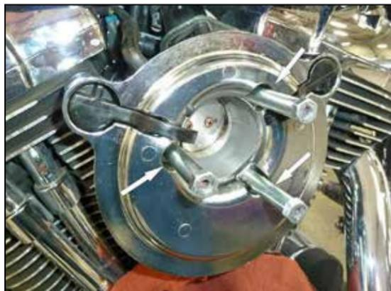
4. Remove the three back plate retaining bolts shown.
