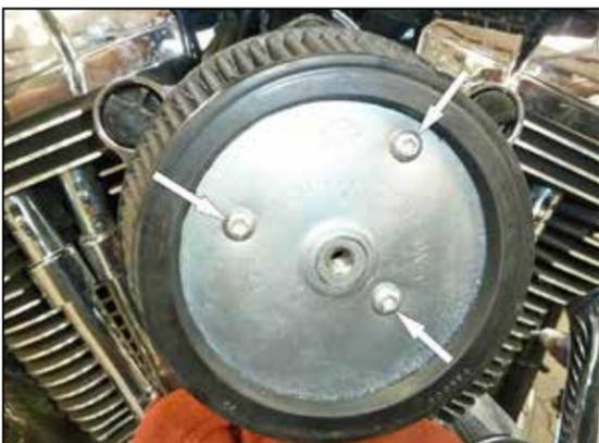
3. Remove the three Torx screws that attach the air filter.
