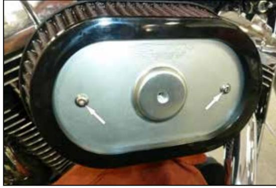
11. Place the K&N® filter on the back plate and attach with the remaining button head screws.
