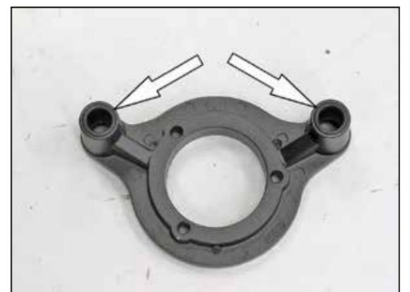
6. Install two of the provided O-Rings into the K&N® throttle body bracket as shown.
