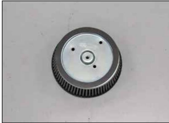
9. Install the provided gasket onto the K&N® air filter as shown.
