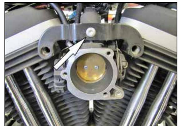
5. Remove the bolt securing the throttle body bracket and then remove the throttle body bracket from the vehicle.
