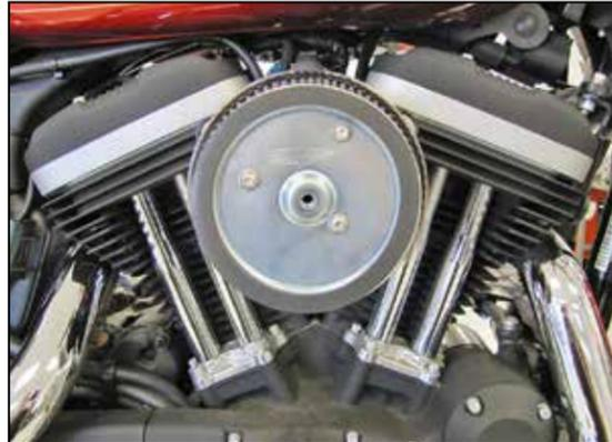
10. Install the K&N® air filter onto the back plate and secure with the provided hardware.
